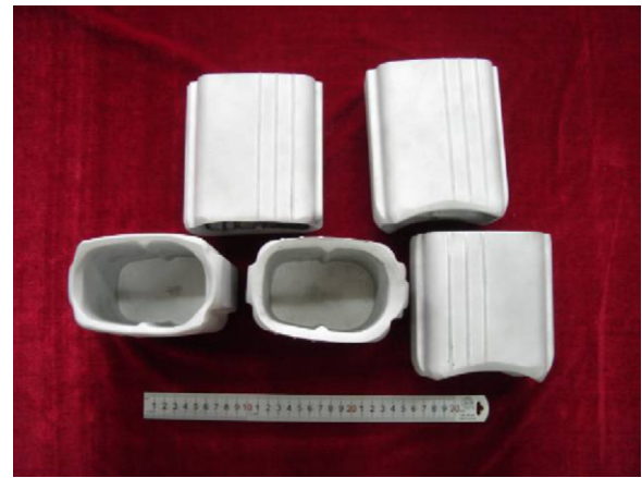
Fig. 19. Barrel-shaped components thixoextruded from eight-pass RUE formed AZ80 magnesium alloy.
